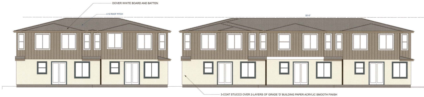
REAR ELEVATION UNITS 'B'
