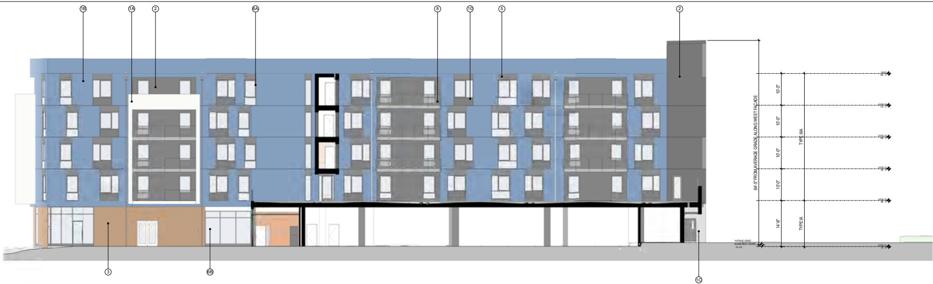
1 NORTH ELEVATION - AT FORECOURT/COURTYARD 1/8" = 1'-0"
