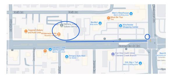
One other suggestion was having Mission Trail trucks enter the Subaru property from Stevens Creek to collect waste internally. This suggestion is not feasible. The dealership's fire suppression system imposes a low clearance that prevents truck access. Additionally, the property layout would require trucks to reverse back onto Stevens Creek Boulevard or Cecil Avenue, introducing new safety risks, increased noise pollution, and greater disruption to traffic.
