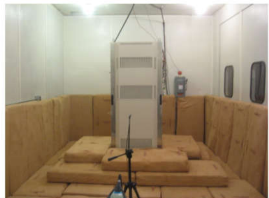
Figure 9.1a: Acoustic Test at 0°
