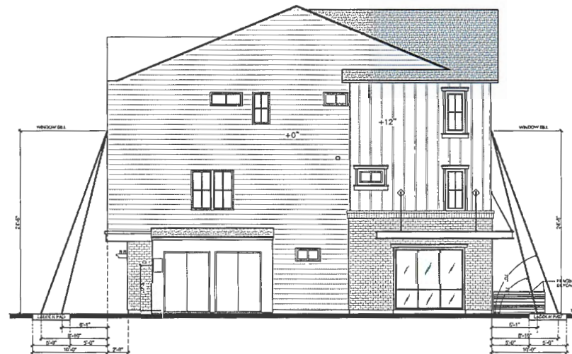
TYPICAL DIAGRAM LADDER PAD LOCATION FOR CATALINA II SIMILAR CONDITION FOR ALL BUILDING TYPES INCLUDING LIVE/WORK
