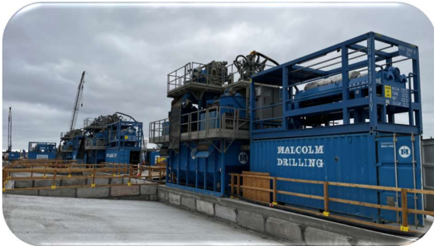
Slurry Wall Desander Equipment – Used to Separate Soil from Slurry
