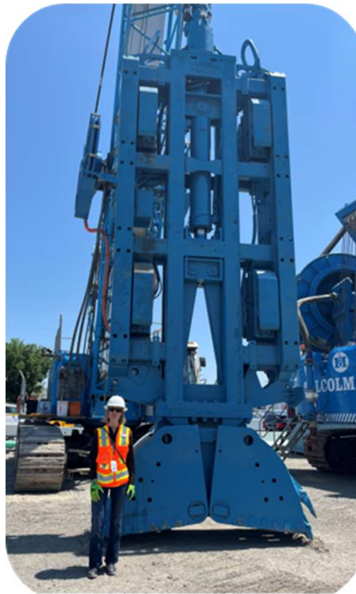
Slurry Wall Drilling Equipment – Hydromill Used to Excavate Materials
