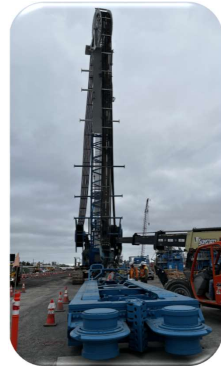
Slurry Wall Drilling Equipment – Hydromill Used to Excavate Materials
