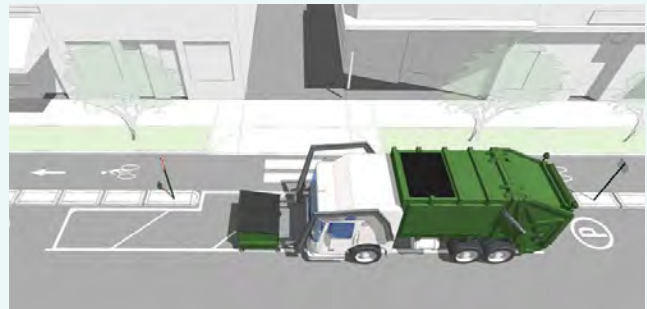
Loading and Garbage Access at Mid-Block Locations (Source: 2017 Fresno Class IV Bikeway Design Guide)
