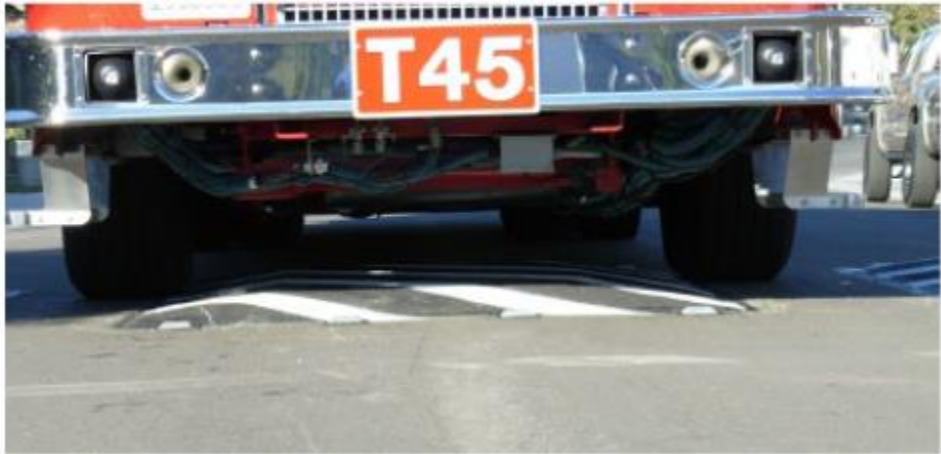
Fire truck driving over speed cushion
