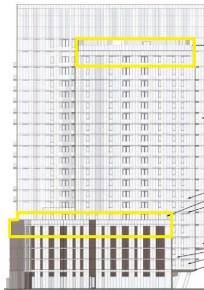
Figure 13. On the building's west façade, areas above and below terraces with landscape vegetation are outlined in yellow. These areas should be treated with a bird-safe glazing treatment.
