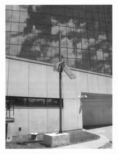
Each noise monitoring station will include a noise sensor, a digital noise logger, and a cellular modem for automatic remote data transmission (24/7). Additional information about the Seti-Media noise monitoring stations may be found in the appendix.
