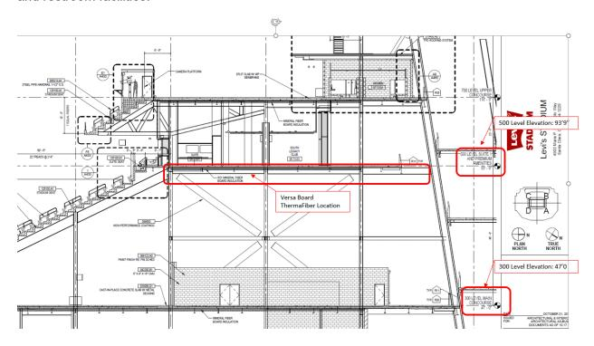
Layout drawing shown below to represent area of Capping installation (shown in purple) above concourse, concession and restroom facilities.
