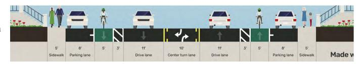
Four Lanes, Buffered Bike Lanes, Remove Parking on One Side
