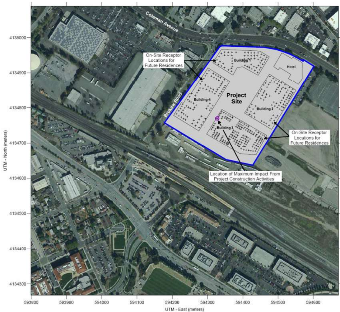
Figure 2. Project Construction Site and Locations of On-Site Sensitive Receptors and Maximum TAC and PM 2.5 Impacts
