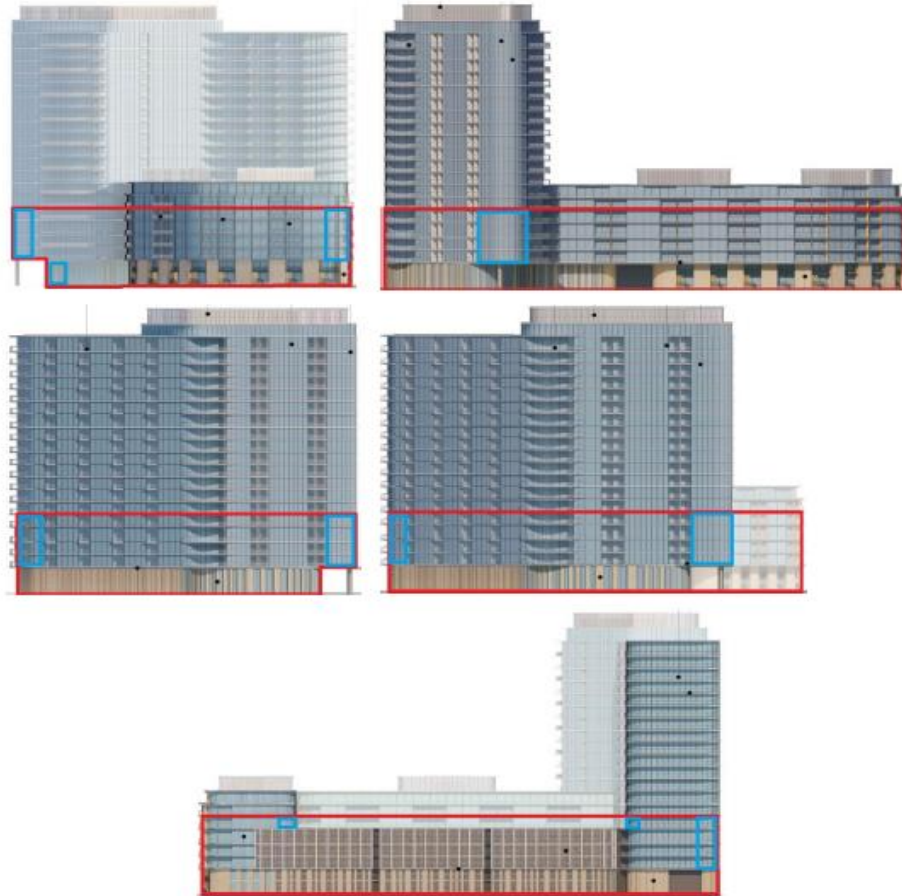
Figure 7. The north (top left), east (top right), south short (middle left), south long (middle right), and west (bottom) facades of Building 4B. Areas outlined in red shall be treated with a bird-safe glazing treatment such that no more than 10% of the façade areas (combined) consists of untreated glazing. Areas outlined in blue (transparent glass corners) shall be 100% treated with a bird-safe glazing treatment.
