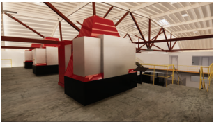
P4 - ROBOTICALLY FED 5-AXIS LATHE ARRAY - BUILDING 'X'
