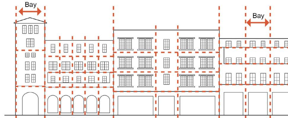
*Facade elements shall be organized by a grid. Rooflines, openings, and other materials must align horizontally. Facade elements or massing increments shall be divided into vertical bays.*
