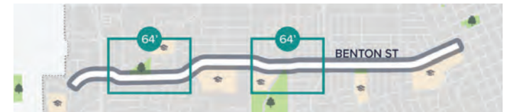
BUFFERED BIKE LANES A buffer between vehicle traffic provides additional horizontal separation from vehicles.
