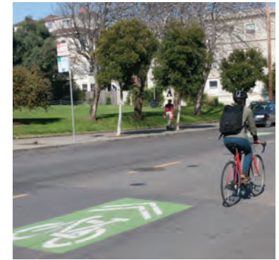
BIKE BOULEVARD Bike boulevards share roadway priority with cyclists. Traffic calming elements may be introduced to deter excess vehicle speeds for comfort and safety on the shared roadway.
