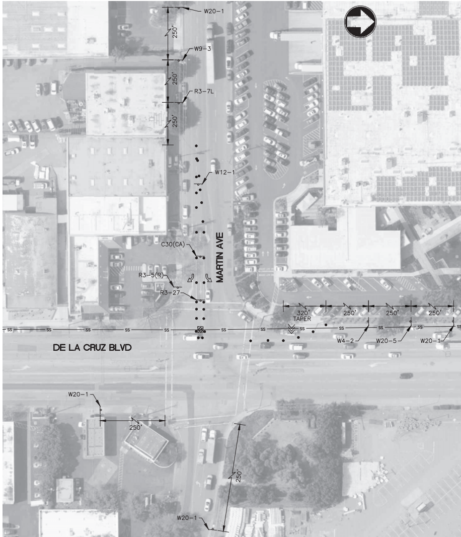
TRAFFIC CONTROL MEASURE #1: CURED-IN-PLACE PIPE AT INTERSECTION OF DE LA CRUZ BLVD AND MARTIN AVE
