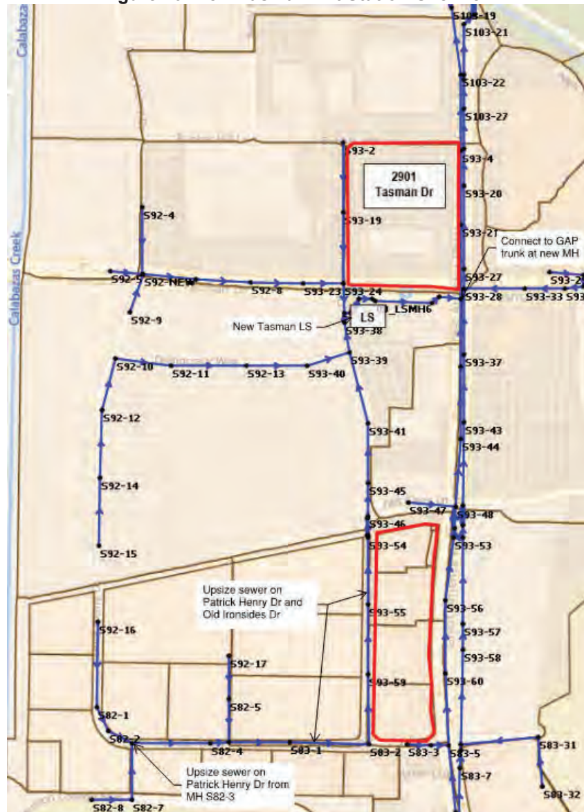
Figure 10: New Tasman Lift Station Overview
