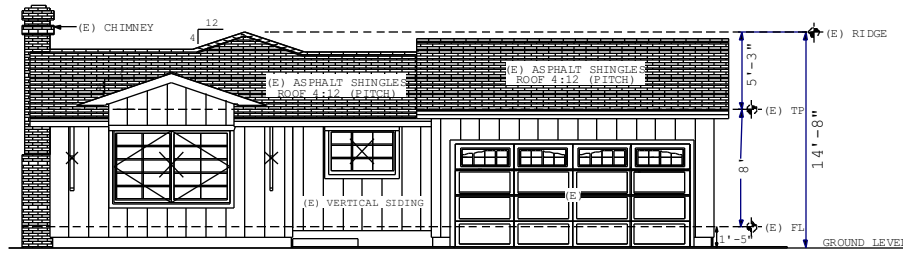
EXISTING FRONT ELEVATION 1/4" = 1'-0"
