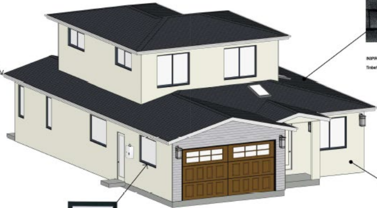
James Hardie Soft Fiber Cement Vented Smooth Panel painted black satin finish 2X10 FASCIA JAMES HARDIE - WITH ROYAL MOLDING
