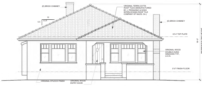
EXISTING FRONT ELEVATION
