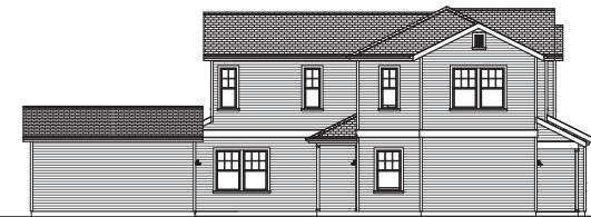
Architectural drawing of the East Elevation of a two-story house. The drawing includes a garage on the left, a central entry door, and several windows. Annotations specify materials: ROOF = CERTAINTIED 40 YEAR COMP SHINGLE, TIMBERLINE HD WEATHERED WOOD HARDI-PLANK SIDING = SHERWIN-WILLIAMS 7641 COLONNADE GRAY WINDOWS = ANDERSON 100 SERIES, WHITE WINDOW, DOOR TRIM & EAVES = SHERWIN-WILLIAMS 6365 DOVER WHITE ENTRY DOOR = SHERWIN-WILLIAMS 7591 RED BARN HARDI-PLANK SHINGLES EAST ELEVATION
