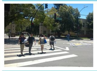
Leading Pedestrian Intervals are pedestrian-only crossing signals that occur slightly before the green signal for parallel lanes of vehicle traffic. They allow pedestrians to get a head-start in the crosswalk, making them more visible to turning motorists.
