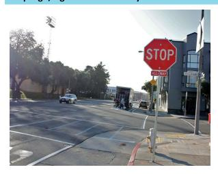
Stop Sign or Signal Warrant Studies evaluate whether there is sufficient vehicle or pedestrian volumes at an intersection to warrant the installation of traffic controls. Changes in land use can increase traffic volumes, necessitating installation of stop signs or traffic signals.
