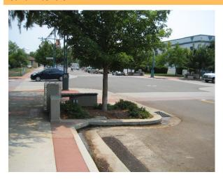
Curb extensions, or bulb outs, are extensions of the sidewalk and curb at the corners of intersections. They shorten the roadway crossing distance and make pedestrians more visible to motorists. They can also help calm traffic by narrowing the travel lane, and provide additional space for plantings and street furnishings.
