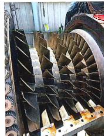
Rotor As-Found. Forward Casing Removed
