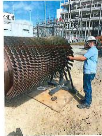
Compressor Rotor Exposed for Inspection
