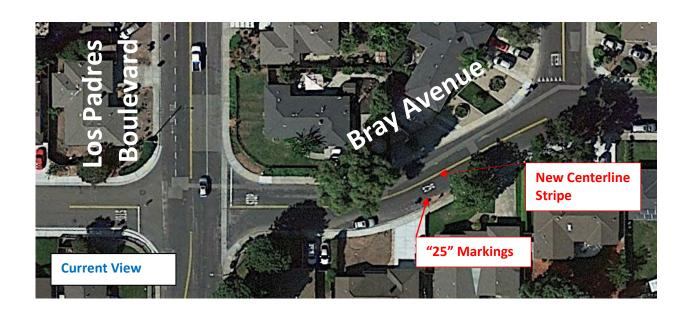
Pictures of "S" Curve Centerline Striping Installation
