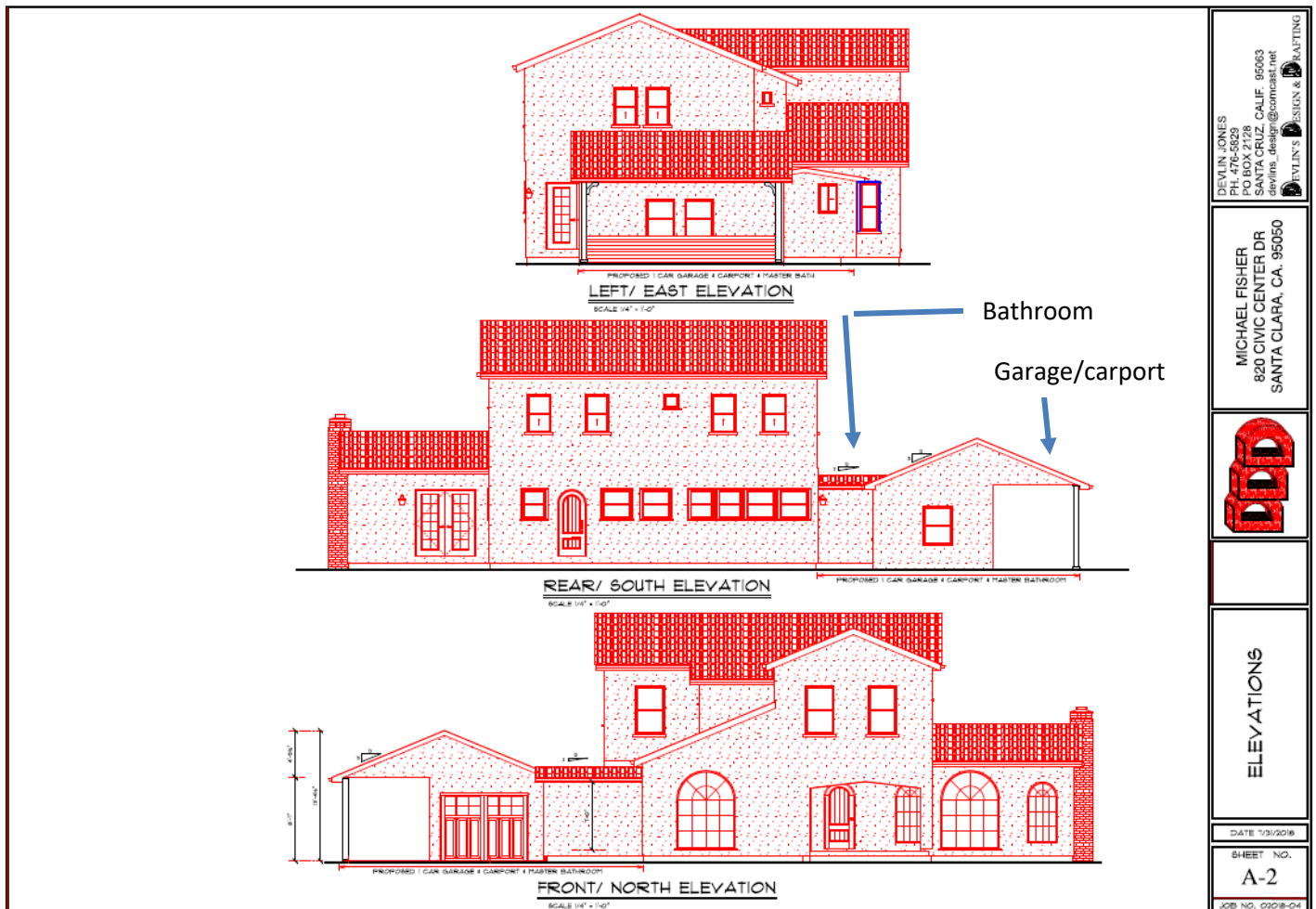
Figure 2 : Sheet of elevations showing the proposed bathroom addition and the new garage and carport. From the side the garage will screen the lower portion of the house. From the rear, the house is not visible and the new garage/carport will be only slightly visible from Alviso St. From the front the garage/carport is seen set back from the house as a separate structure. The bathroom set back from the front façade of the historic house and is attached to the historic house. This is a minor addition, on a secondary façade and will be covered with plain stucco and roof tiles that are similar to the historic building. The small addition is designed to be compatible with the front view of the historic house.
