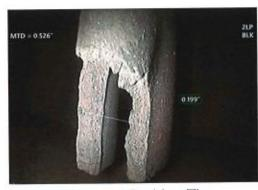
**Damaged Turbine Tip**
