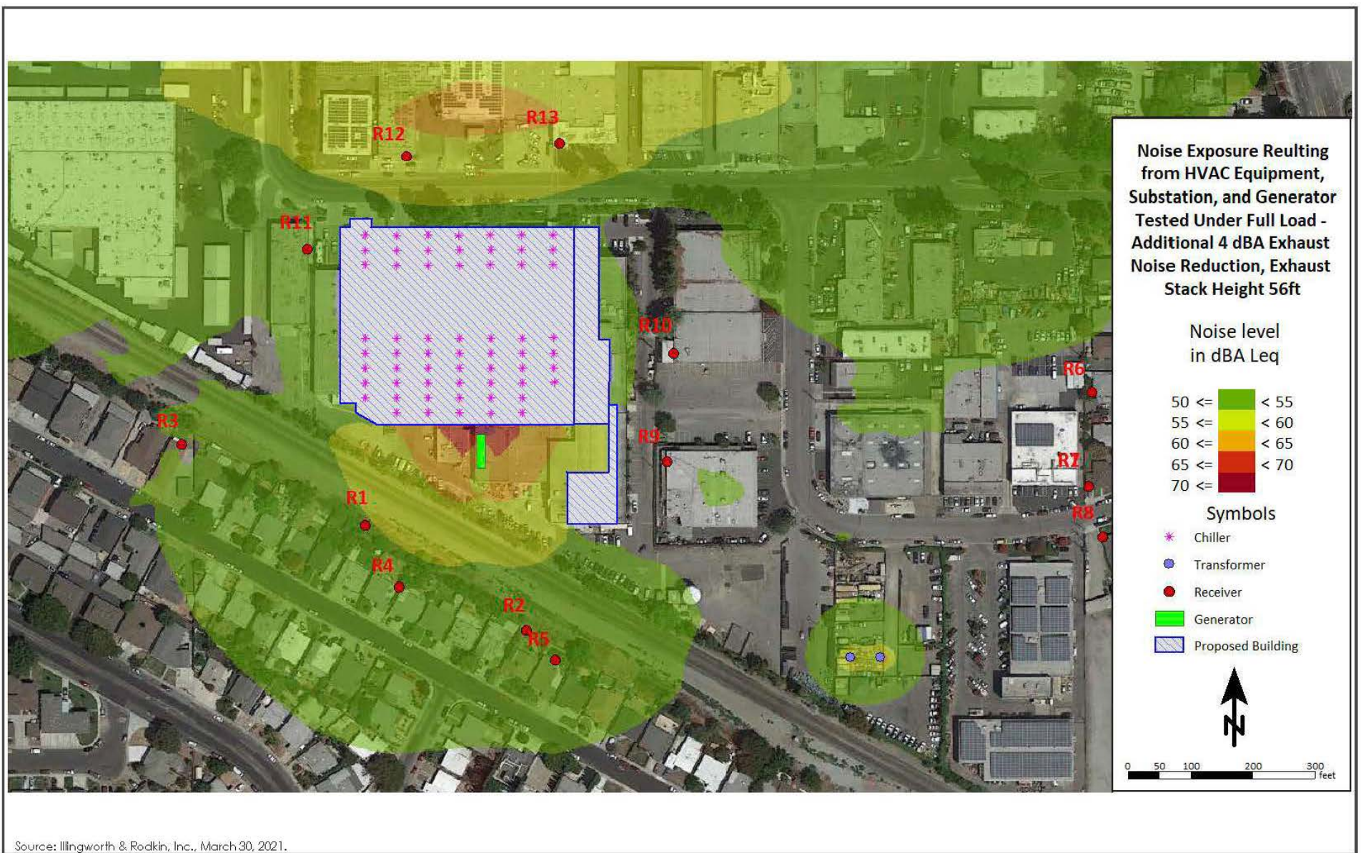
NOISE EXPOSURE RESULTING FROM HVAC EQUIPMENT, SUBSTATION, AND SINGLE GENERATOR TESTED UNDER FULL LOAD
